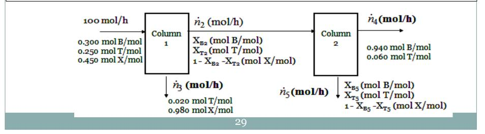
(a) Draw and label flowchart. Do the degree-of-freedom analysis to prove that for an assumed basis of calculation, molar flowrate and compositions of all process streams can be calculated from the given information.
