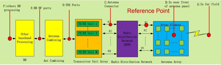
Massive MIMO Structure and Different Test Reference Points
