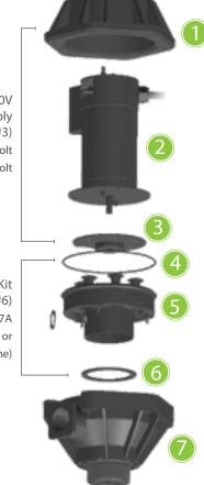
12V or 110V Motor Assembly (#1 - #3) DP-P4012-M 12 Volt DP-P4015-M 110 Volt
