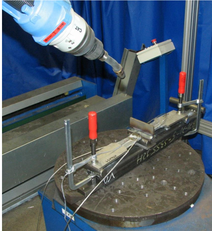
Figure 12 Experimental setup for welding the specimen mounted with gauges and thermocouples
