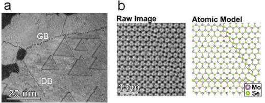
Figure 1: Aberration-corrected transmission electron microscopy (AC-TEM) image of a MoSe2 layer; (a) overview of grain and inversion domain boundaries and b) atomic structural analysis of inversion domain boundary [2].
