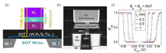
Figure 1: a) schematic of SOT-MTJ, and possibilities to assist it with STT and VCMA effects, b) TEM Cross section of a SOT-MTJ produced at IMEC [4], c) typically switching probability as a function of SOT voltage operated at 0 external field [4].
