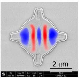
Figure 1: SEM image of a suspended drum-like YIG resonator with an overlay of a spin wave pattern measured on the same structure by TR-MOKE.
