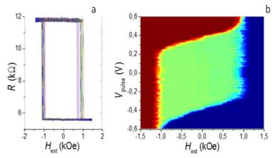
Figure 1: a) A Magneto-Resistive (MR) hysteresis cycle measured on a perpendicular anisotropy tunnel junction showing the variation of the resistance and two distinct resistance sates [1]. b) A state-phase diagram plot of the same junction when applying current pulses. The color code shows the resistance state, blue for low and red for high resistance, with green being the bi-stable region for memory cell.
