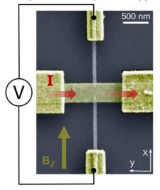
Figure 1 : Example of a nanodevice made in our team allowing the electrical measurement of the charge current - spin current conversion [4]. The charge current travels along the horizontal track in the spin-orbit material, generating a spin accumulation, and the vertical ferromagnetic electrodes probe this accumulation.
