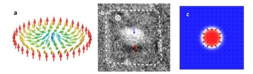
Figure 1: a) Schematic representation of a magnetic skyrmion [1]. b) XMCD-PEEM image of magnetic skyrmion (130 nm diameter) at room temperature and zero magnetic film in an ultrathin Pt/Co/MgO nanostructures [3]. c) Spin structure from micromagnetic simulations.
