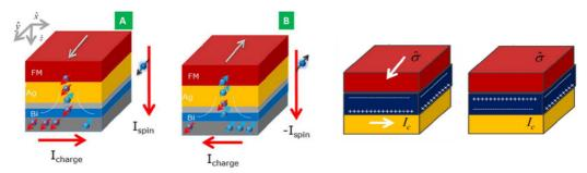
Figure 1: Spintronics devices associating two types of components : ISHE/Rashba metallic pillars converting vertical spin current into horizontal charge current (left) and Magnetoelectric insulating capacitors allowing to switch the magnetization of nanomagnets (right)
