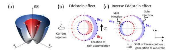
Figure 1: a) Band structure of a Rashba system, with two Fermi contours having opposite spin helicities. Charge-spin (b) and spin-charge (c) conversion: in (b) the injection of a charge current  $J_c$  along y shifts the Fermi contours and generate a spin-density  $\sigma = \& \uparrow \& \downarrow$  along x. In (c) the injection of a spin density  $\sigma$  along x shifts the contours along y, creating a finite charge current.
