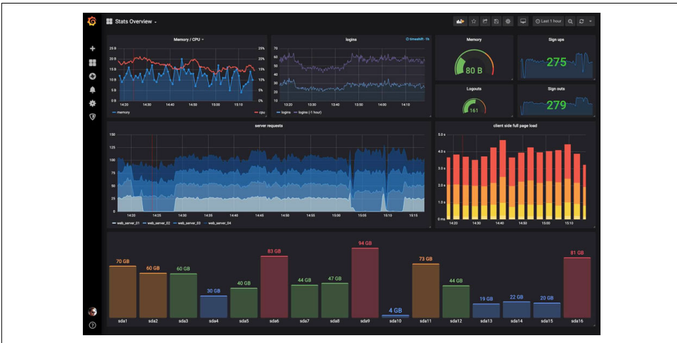
Figure 12-7. The Grafana dashboard utilizes summaries, gauges, histograms, and counters to visualize metrics from a time series database.
