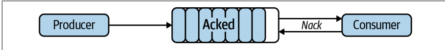
Figure 5-23. A consumer negatively acknowledges the latest message in the subscription. Unlike all other messages in the subscription, this message is treated as if it wasn't ever sent to the consumer.
