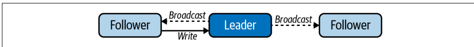
Figure 4-22. The commit protocol used in ZooKeeper is useful as a notification protocol.
