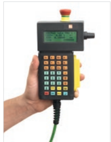
Hand-held keyboard for axis handling in manual mode, necessary when preparing the working area and tooling the machine.
