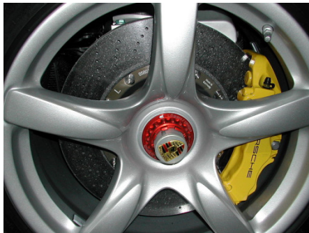
carbon-fiber-reinforced silicon carbide (C/SiC)
