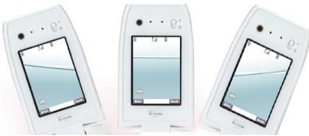
Figure 3. A mobile phone interface where battery level is indicated via the illusion of a water-filled container.
