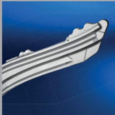
Flap Track 2.450 mm x 630 mm x 160 mm 371 kg
