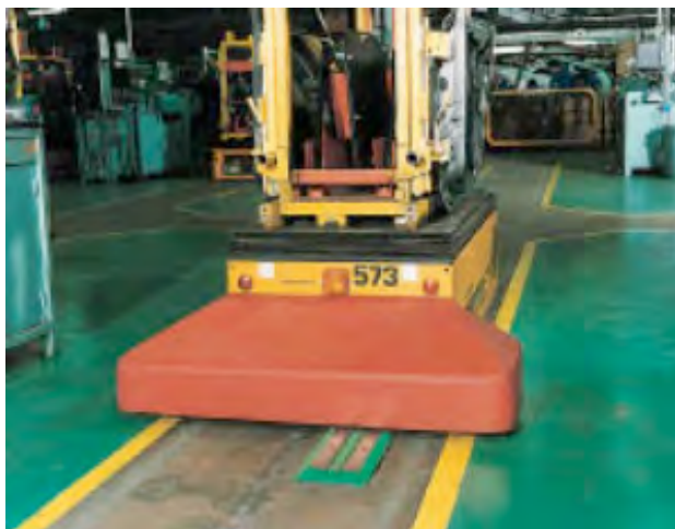
Figure 2. Automatic Guided Vehicle System. This AGVS is guided by a floor path. http://www.vahleinc.com/images/sys_bc.jpg
