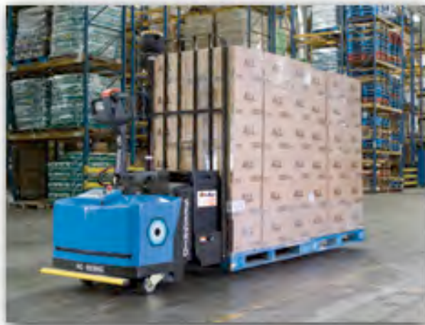
Figure 13. Seegrid G8 pallet truck moving a pallet. This AMR is capable of moving 8,000 pounds. http://www.seegrid.com/index.php
