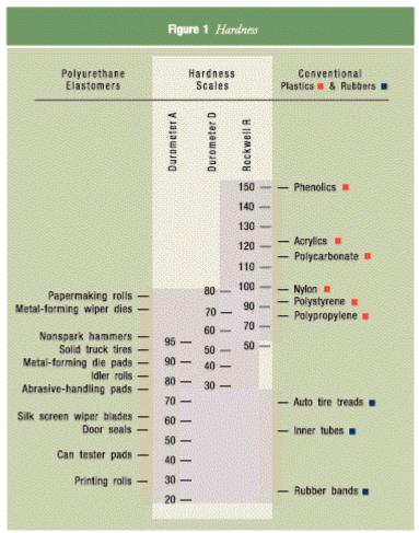
Figure 7. Hardness comparison scale of some materials [17]
