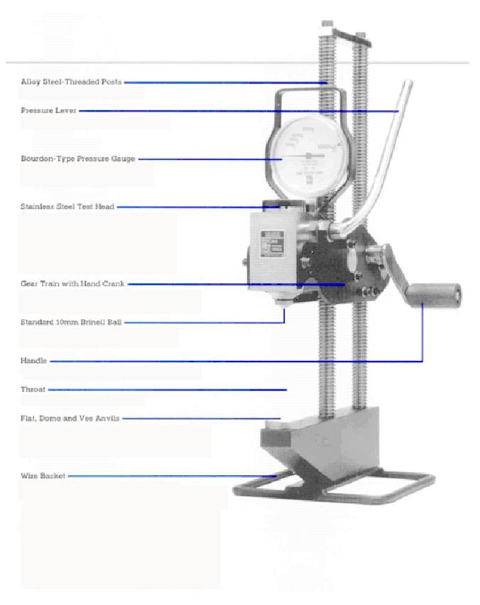
Figure 15. Brinell Hardness Tester
