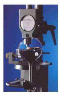
Figure 21. Equipment for hardness determination of Plastics, Elastomers, O-Rings, Seals, Gaskets, Rubber Rollers.
