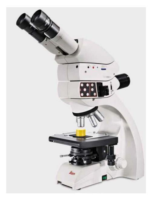
Through sturdy design with LED illumination Accurate analysis results through brilliant Leica HC optics Identification of the finest details through oblique light with LED segmented lighting.
