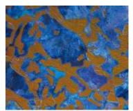
Ferrite C60, hypoeutectoid pearlite, N Plan 50×, Differential interference contrast
