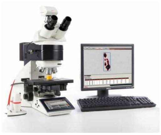
Using the automated image analysis functions of Leica Steel Expert 2.0, both single and multiple samples can be analyzed regardless of your Leica microscope model and degree of automation. Leica Steel Expert 2.0 also enables simultaneous comparison of results in accordance with various existing industry standards – including ASTM E45 A, D, and E, ISO 4967 A and B, DIN 50 602 (K and M methods), EN 10 247, as well as JIS G0555, GB/T 10 561 (in progress).
