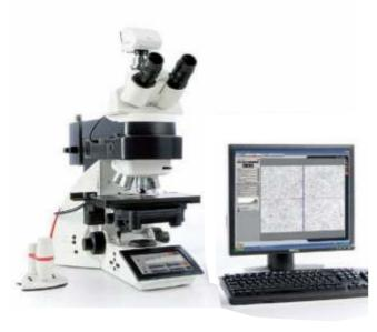
Leica Cleanliness Expert is ideal for all applications involving particle classification and characterization on circular shaped substrates. The software typically supports users in the automotive, galvanic, and aviation sectors, as well as the pharmaceutical industry. It is particularly useful to conduct analyses when hydraulic fluids are concerned.
