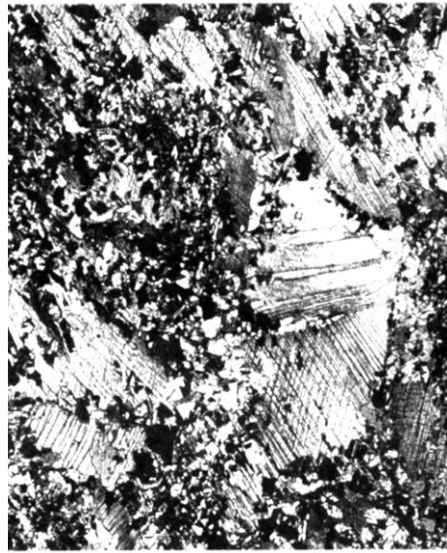
Partial replacement of grains, after 4 seconds
