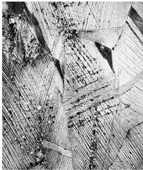
Initial recrystallization after 3 seconds @ 580°C
