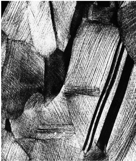
Cold Worked grains. Not annealed.
