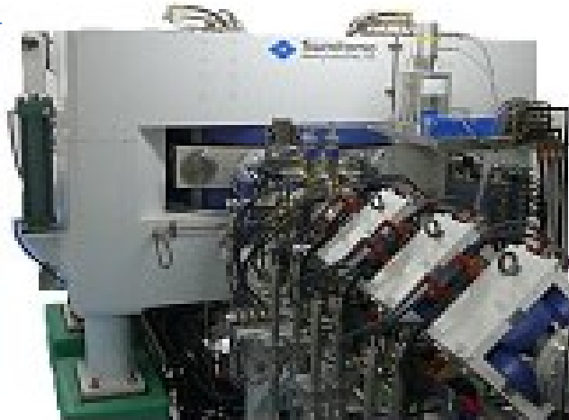
Sumitomi Heavy Industries Cyclotron 18 MeV protons, 50 μA beam current
