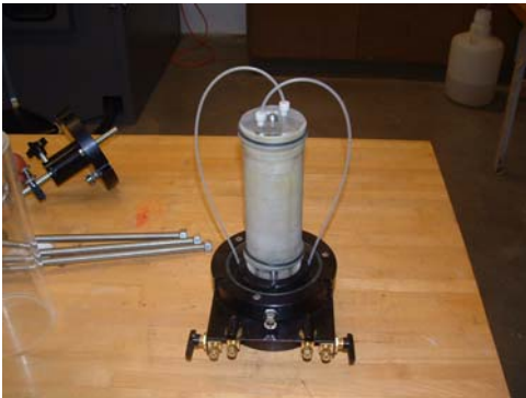
(b) Seating a specimen on the cell base and placing the top cap
