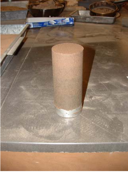
(a) Compacted subgrade soil specimen
