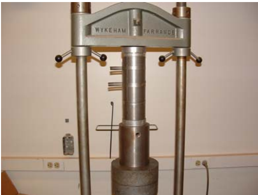
(c) Applying static force to compact soil specimen
