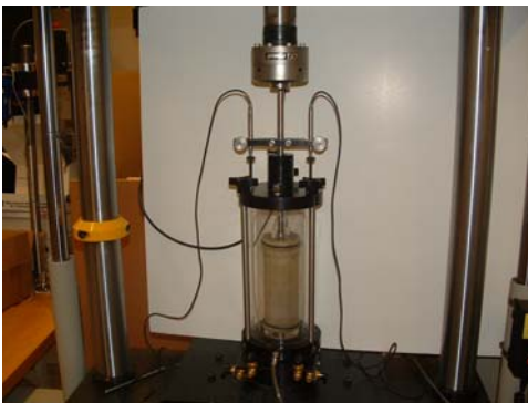
(c) Mounting the cell on the loading frame
