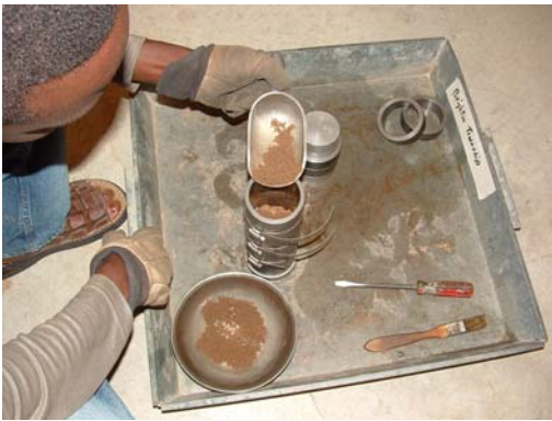
(b) Filling mold with one soil layer
