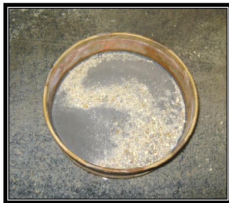
Figure 4 Material Retained on the No. 200 (75 \mu\text{m} ) sieve
