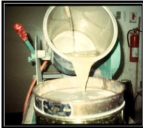
Figure 3 Pouring Water through Sieves
