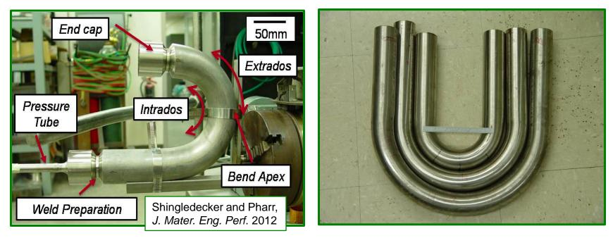
Cold-bent tubes are being creep tested to provide guidance for determining fabrication rules for Ni-base alloys
