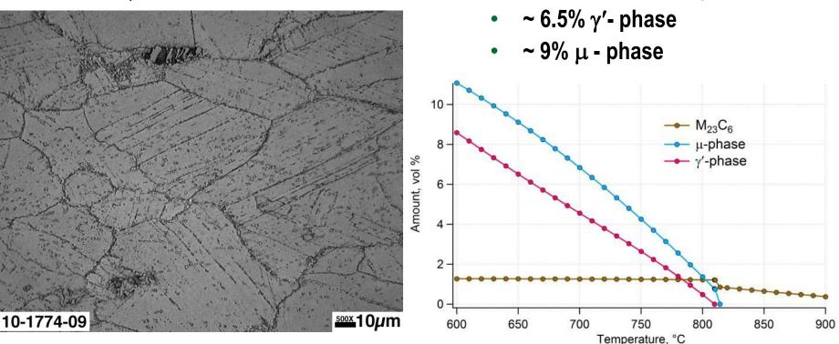
Microstructure analysis for phase identification is in-progress
