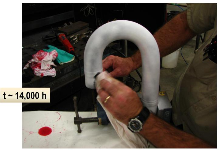
Stains and failure conditions are monitored with periodic shutdowns
