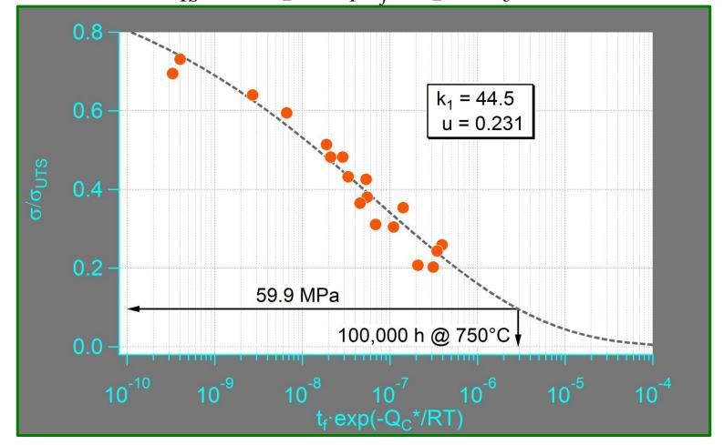
SA vs. aging reduces 100,000 h/750 C creep strength from 105 MPa to 60 MPa
