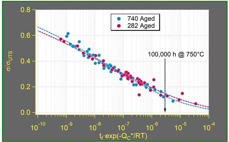
For 100,000 at 750 C, compared to 740 (105 MPa) the higher predicted strength of 282 (128 MPa) is consistent with its higher Mo
