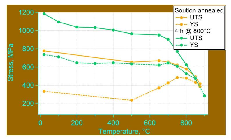
Aged condition maintains advantage over solution annealed until T approaches the  $\gamma'$  solvus (~ 980°C)
