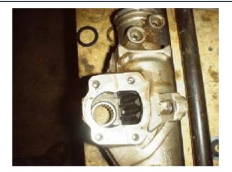
I use an impact socket that is just smaller than the outside bearing diameter. Hit it with a brass mallet or dead blow mallet from the top and drive it out towards the bottom. They usually will come out pretty easy. Take note of the orientation of the sector shaft seal. It will have a clear plastic ring on it that points down and a soft rubber section on the top. There may be a large metal washer on top of the clear plastic ring depending on your box. AGR's will not have the large metal washer.
