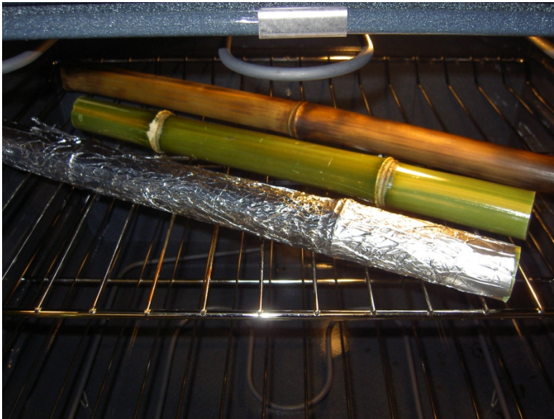
Testing the baking of bamboo with a fresh piece, a piece that was previously blowtorched, and a fresh piece wrapped in aluminum foil.
