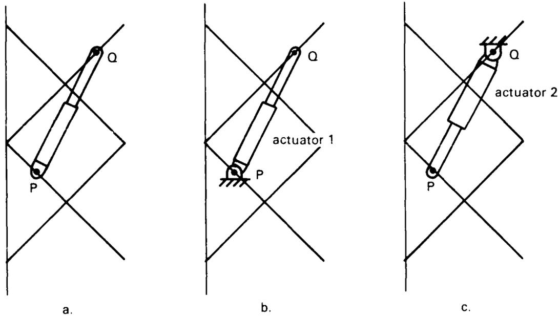
Figure 25. Actuator models.
