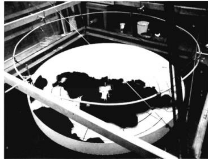
Figure 1. The rotating tank experimental apparatus and wind system is shown. The tank is 2 m in diameter and mounted on an axis which is vertical to 10^{-3} radian. It spins at about 8 rpm during the experiment. The
