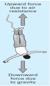
Air resistance can be formulated in a variety of ways. From fluid mechanics a good first approximation would be to assume that it is proportional to the square of the velocity,
