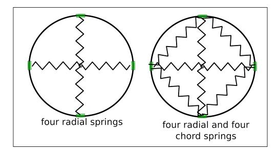
On the left, four identical radial springs are attached to a node and their ends are attached to beads that are free to move on a circular ring. On the right, four additional springs are attached to the beads—these springs have the same spring constant as the radial springs. The ring has radius R.
