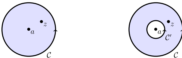
Figure 10: The curves \mathcal{C} and \mathcal{C}' are circles centered at the point a of respective radii R and r < R . The shaded areas are the regions where the function f is holomorphic respectively for the Taylor and Laurent expansions.
