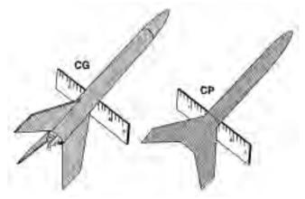
disc or cone for stabilizing, the lateral center of pressure should be set at least 1 1/2 diameters behind the center of gravity.
