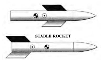
Younger students can be helped to understand the center of pressure by finding the balance point of a number of geographic shapes used in the construction of model rockets. (See Appendix ) This balancing point, referred to as the centroid, describes the geometric center of area for a given shape. The term  $\bar{x}$  locates the centroid from a reference point.
