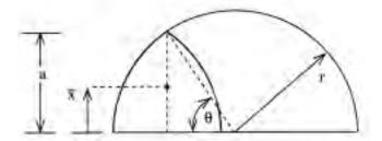
Calculating the center of pressure of rocket outline
