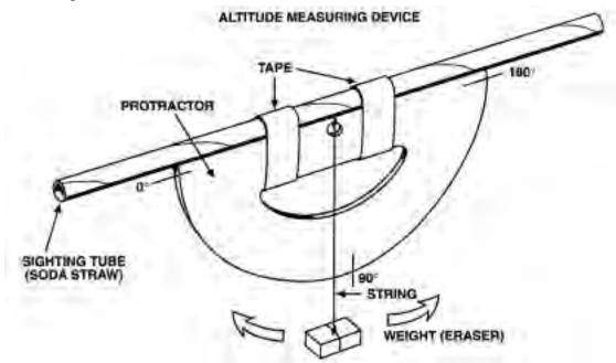
You will be constructing a device that looks like the one in the diagram. Tape the straw across the top of the protractor as shown. The straw will act as a sighting tube. Secure the string to the protractor by slipping it under the straw and around. Tie it to itself and tape it to the back of the protractor. Tie the eraser at the opposite end of the string so that it can act as a weight.
