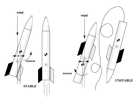
gravity. When it turns, the air rushing past it will then hit the rocket at an angle. If the center of pressure is behind the center of gravity on the model, the air pressure will exert the greatest force against the
