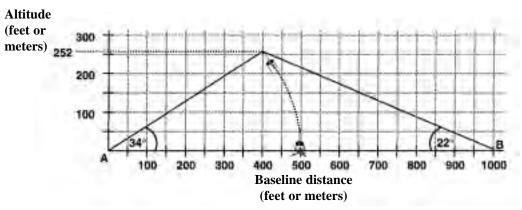
Plot elevation angles A and B, then extend them until they intersect. The point of intersection extended to the vertical axis is the rocket's altitude.
