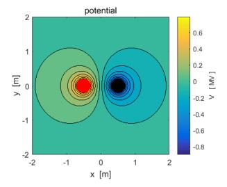
The closer the spacing of the potential contours the greater the electric field strength  $\vec{E} = -\nabla V = -\left(\frac{\partial V}{\partial x}\hat{i} + \frac{\partial V}{\partial y}\hat{j}\right)$ .
