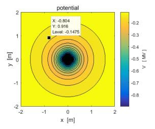
Calculation of the potential between two points by the evaluation of the line integral of the electric field
