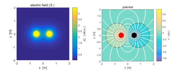
In the plot on the right above, the electric field lines (in white) are superimposed upon the plot of the potential. The direction of the electric field anywhere on an electric field line is from the region of higher potential to lower. It is not so easy to place an arrow on the electric field lines using the Matlab streamline function.
