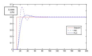
Figure 14: Response of PID & FLC; Vs Time (Sec), for SP=0.5
