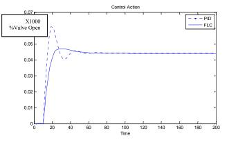
Figure 15: Control Action of PID & FLC; Vs Time (Sec), for SP=0.5.
