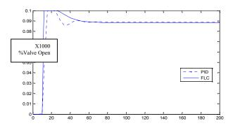
Figure 17: Control Action of PID & FLC; Vs Time (Sec), for SP=1(on Y-axis: 100% valve open is Upper Limit).
