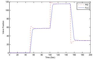
Figure 19: Control action of FLC&PID; Vs Time (sec), SP1=0, SP2=500, SP3=1000, SP4=250.
