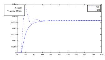
Figure 13: Control Action of PID & FLC; Vs Time (Sec), for SP=0.3.
