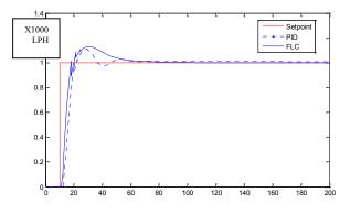
Figure 16: Response of PID & FLC; Vs Time (Sec), for SP=1
