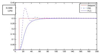
Figure 12: Response of PID & FLC; Vs Time (Sec), for SP=0
