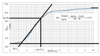
Figure 8: Step response in flow rate for input step change from 40 - 60%.
