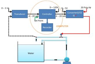
Figure 3.1: Schematic diagram of Flow Process Station
