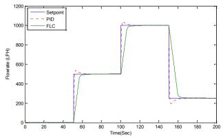
Figure 18: Response of FLC&PID; Flow Rate (LPH) Vs Time (sec), SP1=0, SP2=500, SP3=1000, SP4=250.
