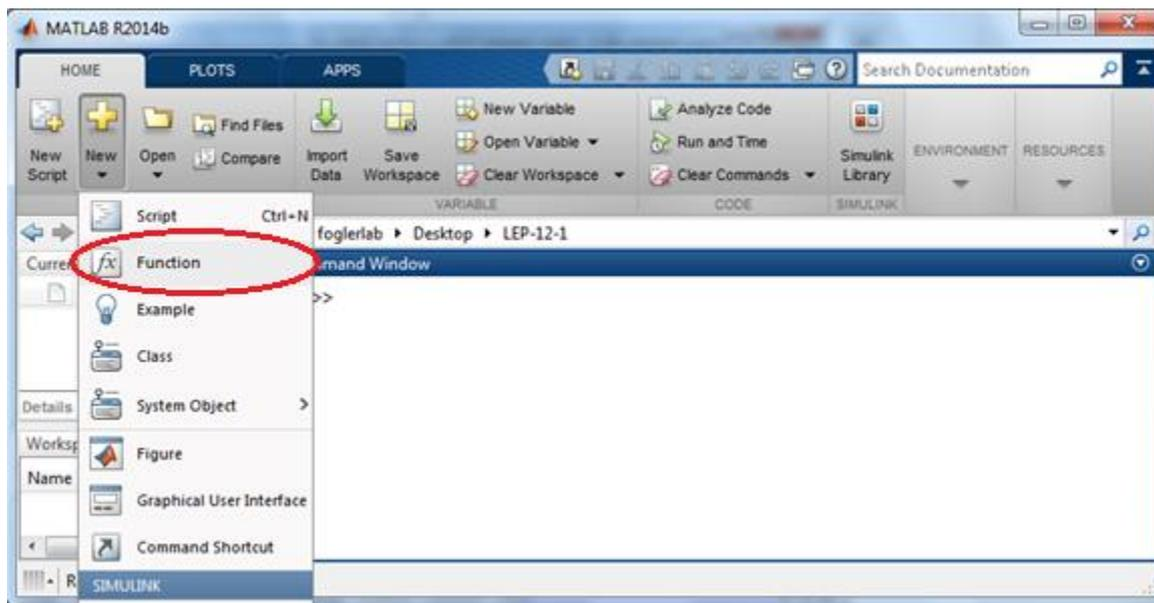
You will see a new window opens that looks like this. MATLAB automatically creates syntax for writing function file. To use solver in MATLAB, you need to write codes in the space provided.
