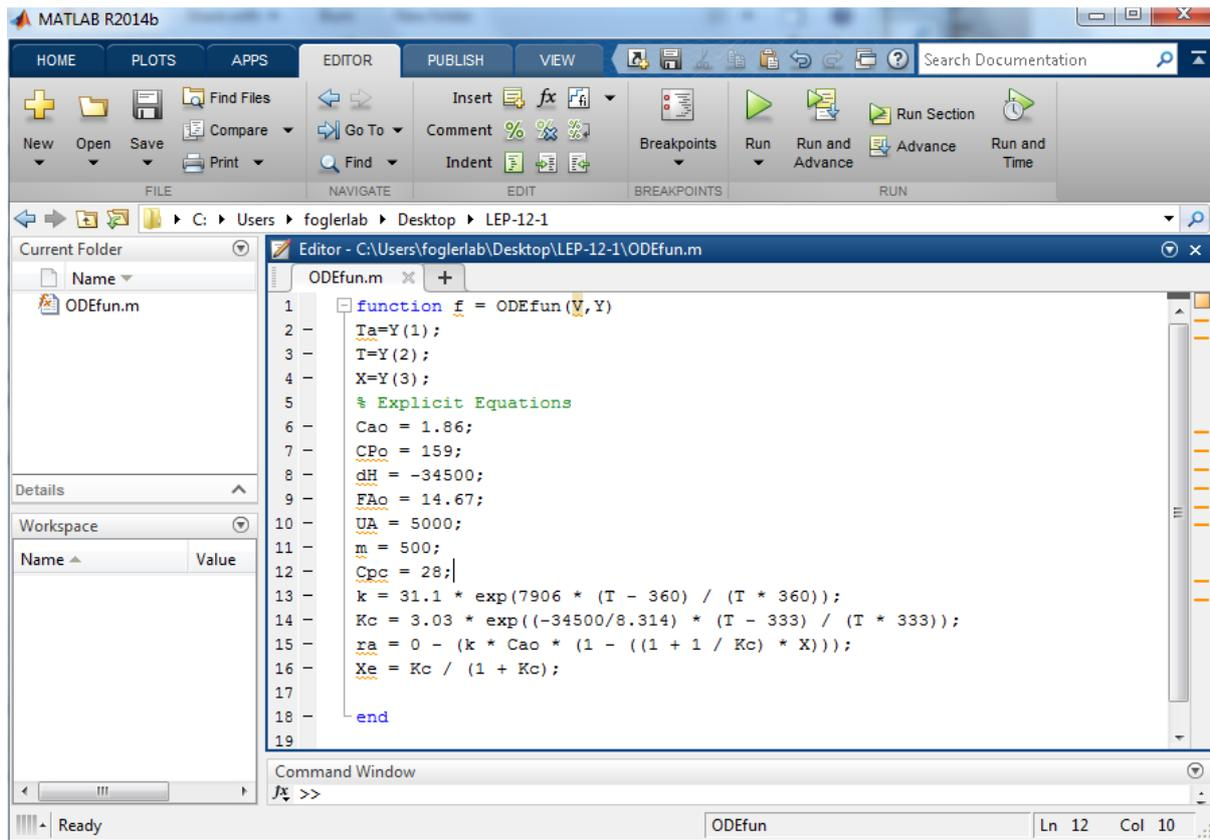
**Step 9:** Next, you need to enter your differential equations. For this example, you have three differential equation in Ta, T and X.
