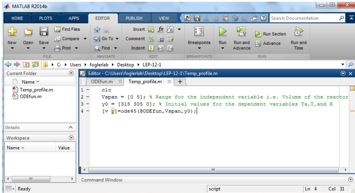
When you run the script file, it will call function file and evaluate the differential equation for different values of independent variable and the output will be stored in [v y]. As described earlier, v is a column vector of volume and y is a column vector of [T, Ta, X]. We will not run the script file at this moment.
