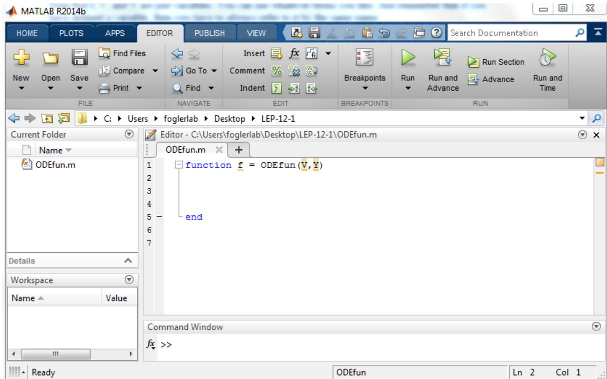
**Step 6:** As the differential equation contains 3 dependent variables (Ta, T, & X), so Y vector contains initial values of these 3 variables, where, Ta is the first element, T is the second element and X is the third element of Y vector
