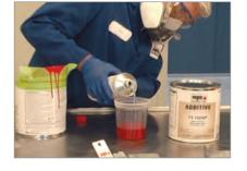
the unit to be painted. Reducers are made up of a combination of fast, medium and slow evaporating solvents. These are blended together to give a reducer a temperature "range" to work within.
