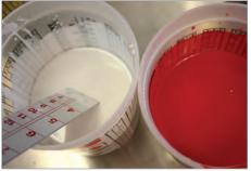
• For especially hot/humid climates, keep the mix room as cool as possible to help keep the toners from drying out. Once the toner loses too much solvent its weight changes and can possibly compromise the color match.
