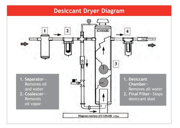
Silica Gel desiccant has been determined to work well in a paint shop but it requires good oil and particle filters and you must regenerate or discard media.
