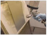
spray pattern not only involves the fluid nozzle adjustment but also the pressure of the atomizing air.
