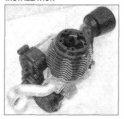
First, remove the engine, installed as standard, with the engine mount.
