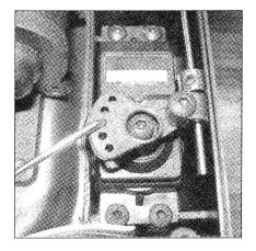
Adjust the aluminum stopper end so that the throttle linkage may be made correctly.
