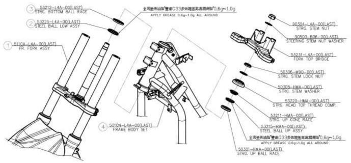
Fig.1 Steering system components.
