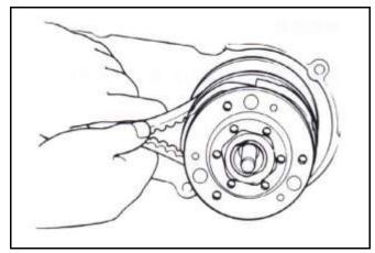
Install the clutch outer and bearing stay collar. Hold the clutch outer whit universal holder, and then tighten nut to specified torque value.
