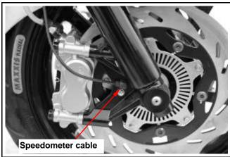
Pull out the front wheel axle. Remove the front wheel and both side collar.
