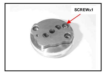
Tighten screw Make sure that oil pump shaft can be rotated freely.
