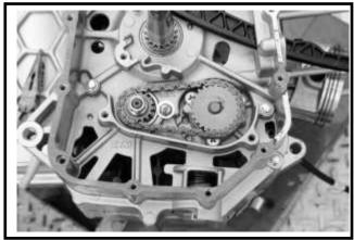
Remove 3 bolts on the oil pump, and then remove oil pump.
