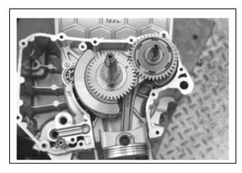
Remove the crankshaft and balancer shaft from the left crankcase.
