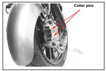
Remove the brake pad shafts and pads.
