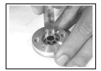
Check clearance between inner and outer rotors.
