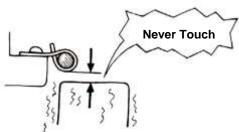
Route wire harnesses to avoid sharp edges or corners and also avoid the projected ends of bolts and screws.
