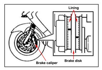
Remove the brake clipper bolt, and take out the clipper.
