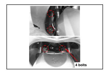
Loosen 2 screws and 2 bolts from the front cover upper side.
