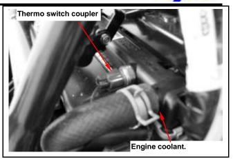
Remove reserve tank coolant inlet pipe. Remove the radiator and the cooling fun.
