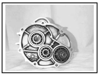
Install the driving shaft onto gear box cover and then place it to proper position.
