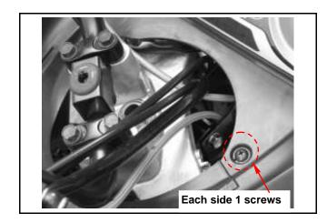
Loosen 2 screws from in side of meter panel.
