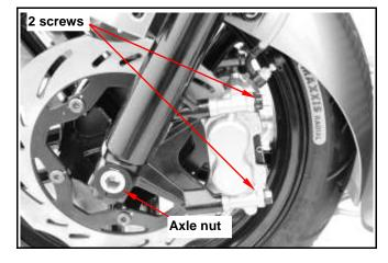
Loosen screw & remove speedometer cable. Turn loose the axle nut.
