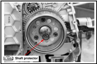
Pull out flywheel with A.C.G. flywheel puller. **Tool:**
