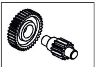
Check if the final shaft and gear are burn, wear or damage.
