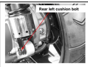
Remove the engine hanger lock nut. Remove the engine hanger axle. Remove the engine.
