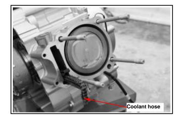
Cover the holes of crankcase and cam chain with a piece of cloth.
