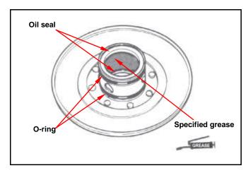
Install the movable driven face onto driven face. Install the guide pin and guide pin roller.
