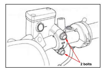
Connect brake hoses with 2 new washers. Tighten the brake hose bolt to the specified torque
