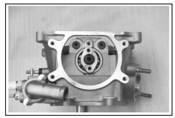
Remove cam shafts.
