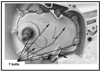
Remove drive shaft. Remove final driving gear and shaft. Remove countershaft and gear.
