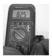
B phase measurement of the resistance value
