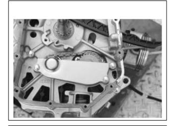
Tighten the bolts on the left crankcase (bolt x 11).
