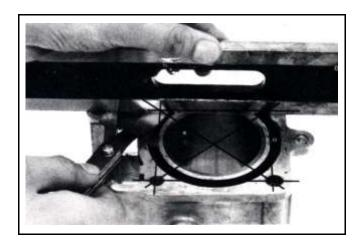
Measure the clearance between piston rings and ring grooves.
