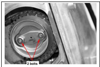
Remove the 2 cylinder head mounting bolts from cylinder head right side, and then remove 4 nuts and washers from cylinder head upper side. Remove the cylinder head.
