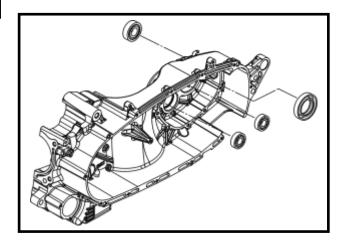
Install new driving shaft bearing into left crankcase.
