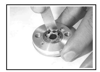
Check clearance between rotor side face and pump body
