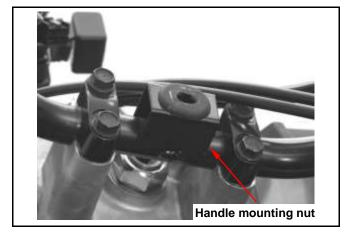
Apply grease to throttle cable and the sliding surface of handle.
