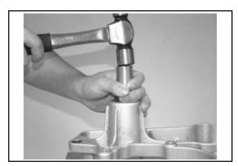
Install new rear fork bearing and bearing puller (6303) onto rear fork.
