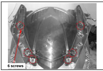
Loosen 4 screws from the meter visor and remove the meter visor.
