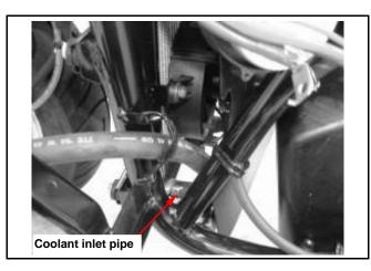
Loosen the cooling fun mounting bolts (3 bolts). Remove thermo switch.
