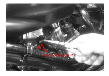
5: Based on the above steps, coolant could be drained out.
