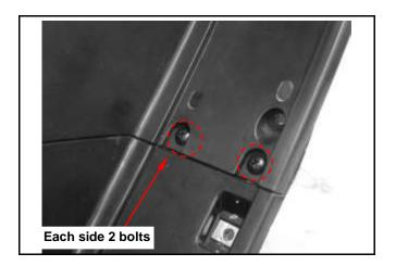
Loosen 2 bolts from inside of the inner box. Disconnect the hazard light and foggy light switch couplers.
