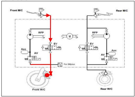
When the brake is applied, speed sensors detect the front and rear wheel speed. When there is no wheel slip, EV (inlet valve for maintaining pressure) keeps open and AV (outlet valve for pressure reduction) is closed. Brake calipers receive pressure for master cylinders and brake normally.
