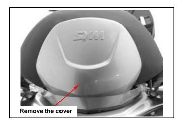
Loosen right, left side and middle screws from rear side of the body cover.
