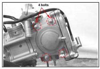
Remove left crankcase cover, and turn the drive face, and align the timing mark on the cam sprocket with that of cylinder head, piston is at TDC position.
