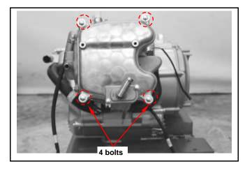
Install Air Injection system (AI) pipe. (4 bolts) Install inlet pipe onto cylinder head. Install and tighten spark plug.
