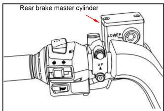
Remove the master cylinder cap and diaphragm. Fill high quality brake fluid with same brand into master cylinder.
