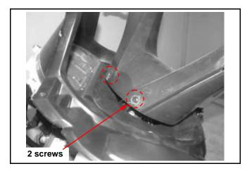
Loosen the 2 screws from handle upper cover rear end.
