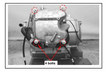
Remove the cylinder head side cover.
