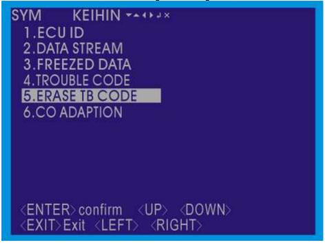
Fault code removed, namely showing the "ERASE TB SUCC.!". Press the "EXIT" button, the function can return to the directory screen.
