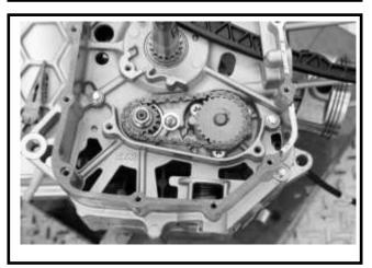
Install starting gear and generator.
