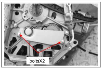
Remove the oil pump drive sprocket, driven sprocket and drive chain.
