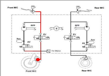
When the initial wheel slip is detected by the wheel speed sensors, EV and AV are both closed. Brake caliper keeps the pressure and brake continues.
