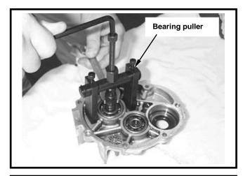
If the driving shaft is pulled out with its bearing, then remove the bearing with bearing puller and bearing protector.
