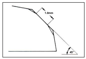
Coat the valve seat surface with red paint. Install the valve through valve guide until the valve contacting with valve seat, slightly press down the valve but do not rotate it so that a seal track will be created on contact surface.
