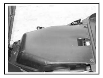
Disconnect the air temperature sensor coupler. Remove the air box.
