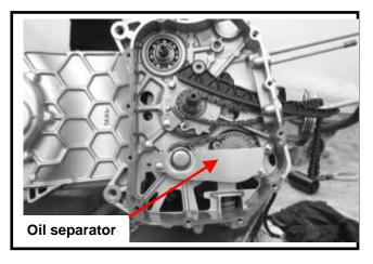
Remove snap ring and take out oil pump driving chain and sprocket.
