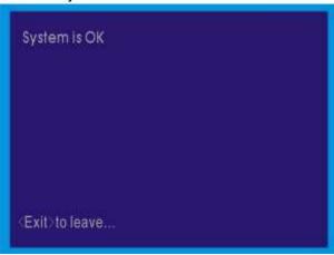
If the system has faulty code, that is showing the fault code, that can be used "◀ left" and "right ▶" or "▲" "▼" button to select the fault code (selected before the code "•" tags) that, press the "ENTER" button, the code can be read descriptions and fault handling.
