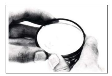
Place piston rings respective into cylinder below 20 mm of cylinder top. In order to keep the piston rings in horizontal level in cylinder, push the rings with piston.
