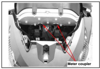
Loosen 4 screws from meter panel. Remove the speedometer.
