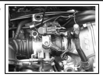
Remove water hose from water pump. Remove the thermo-sensor wires.
