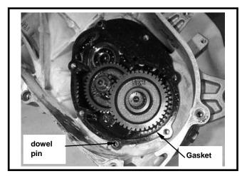
Install gear box cover and bolts, and tighten.
