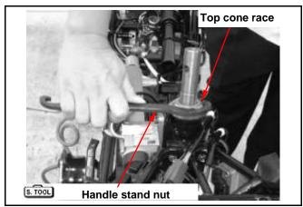
Slightly tap the top and bottom ball bearing seats with a plastic hammer to remove the seats. Remove bottom cone race body with a punch.
