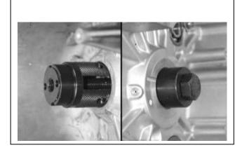
Fix the remover with the universal holder and press out the main bearing.
