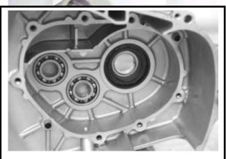
Install countershaft, final shaft and final driving gear.
