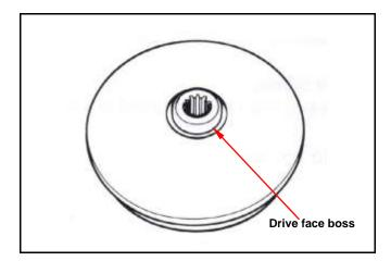
Install movable drive face comp. onto crankshaft.
