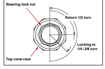
Install the steering stem mounting nut and tighten the nut by means of holding the top cone race body.
