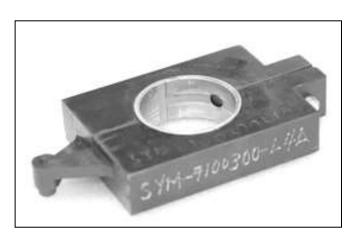
Align the oil path on the main bearing and the crankcase.
