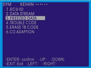
Only one page, at any screen, press the "EXIT" button, the function can return to the directory screen. In the "FREEZED DATA" of the screen use "▲" "▼" button to move the left side of the project "→" symbol selected items, press the "ENTER" button lock of the project, and press the "F4" button showed that the wave of projects.
