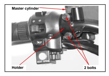
Loosen left handle switch connecter. Loosen 2 screws from left side handle switch holder.
