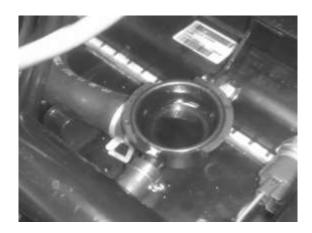
9: Maintain the liquid level in reserve tank between upper and lower limit.
