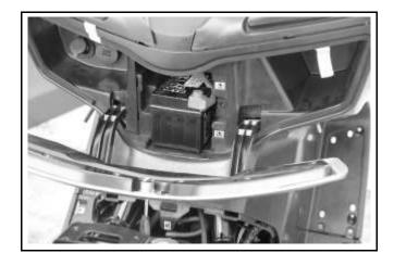
Remove the luggage box. Disconnect the cable positive terminal from the start relay.
