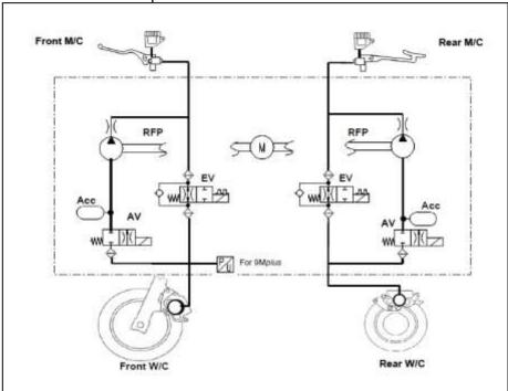
When the wheel speed sensors detect continuous wheel slip, EV keeps closed and AV is open. Brake pressure is reduced (pulsing in the brake lever). Brake caliper lowers the pressure and braking force.
