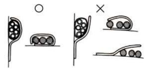
• Do not squeeze wires against the weld or its clamp.
