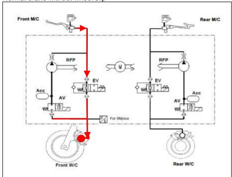
When the pressure reduction continues, the wheel speed sensors detect no wheel slip. EV keeps open and AV is closed. Brake caliper receives pressure from master cylinder and normal brake is applied.
