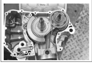
The marks on the crankshaft and balancer shaft must be aligned.
