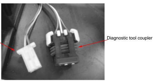
Diagnostic tool coupler and test switch coupler plant
