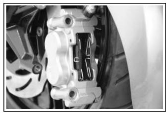
The brake pad must be replaced with new lining when it reaches the wear limit.
