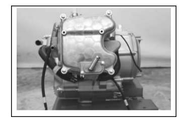
Remove 2 bolts of thermostat and then remove the thermostat.
