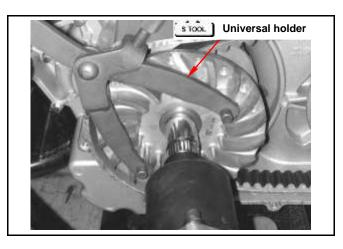
Remove movable drive face comp and drive face boss from crankshaft.
