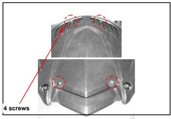
Loosen 4 screws (2 screws on each side) from the inner box.
