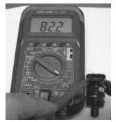
A phase measurement of the resistance value
