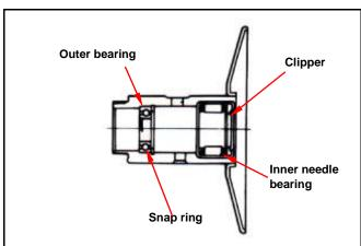
Remove snap ring and then push bearing forward to other side of inner bearing.
