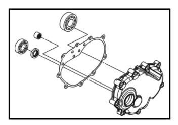
Press out the driving shaft from gear box cover. Using bearing protector as operation.
