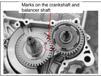
Assemble the right crankcase to the left crankcase.
