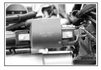
Replacement of ignition coil Remove the cap from the spark plug.
