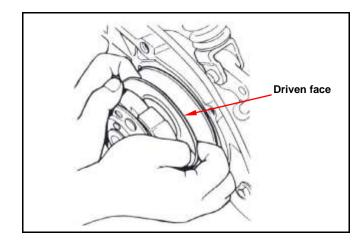
Install the driven pulley that has installed the belt onto drive shaft.
