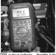
TPS output voltage – throttle fully closed
