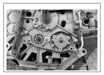
Install the oil pump drive sprocket, driven sprocket and drive chain.
