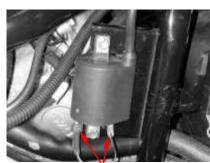
First circuit coil resistance measurement
