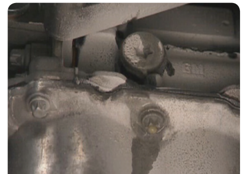
A leak can be traced through the powder back to the source.
