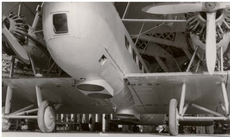
Above and right: Vickers Valentia, K4632, was modified for sky-shouting to marauding Iraqi tribes during air police duties. The installation incorporated four loudspeakers and weighed 1,430lb. RAeS (NAL).
