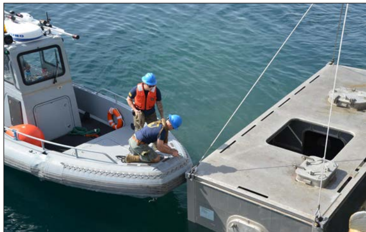
ND2 Aston and ND2 Franklin rigging to transfer the load from the capstan to the crane.
