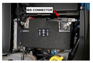
Figure 4 – Battery IBS Connector
