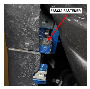
Figure 9 – Fascia to Fender Fasteners
