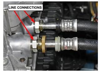
Figure 16 – Connections at Transmission
