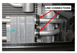
Figure 15 – Transmission Oil Cooler Connections
