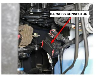
Figure 11 – Wire Harness Connector
