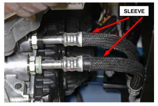
Figure 2 – Oil Cooler Line Sleeve
