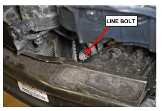
Figure 14 – Oil Cooler Line Brace Bolt
