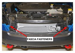
Figure 6 – Fascia Fasteners
