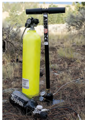
Small-bore air rifles are effectively filled by a hand pump, but large bores are best handled with a scuba tank or small portable tank.
