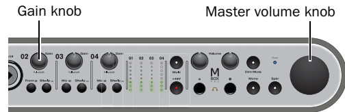
Gain knob for Input 1 (Master volume knob shown)
