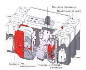
An MCCB provides protection by combining a temperature sensitive device with a current sensitive electromagnetic device. Both these devices act mechanically on the trip mechanism.
