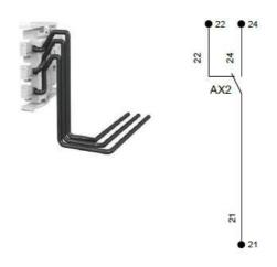
Auxiliary contacts perform the function of electrically signalling the circuit breaker's operating status. The auxiliary contacts change state when the circuit breaker is opened, closed, or tripped.
