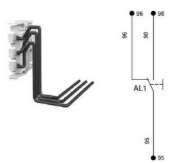
Alarm Contacts (AL) are a special form of auxiliary contacts that indicate the trip status of the MCCB due to:
