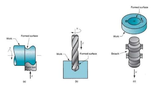
FIGURE 9.3 Forming to create shape in machining: (a) form turning, (b) drilling, and (c) broaching.
