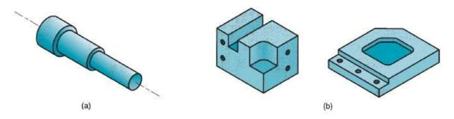
FIGURE 9.1 Machined parts are classified as (a) rotational, or (b) nonrotational, shown here by block and flat parts.
