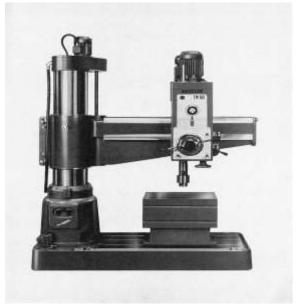
FIGURE 9.11 Radial drill press.
