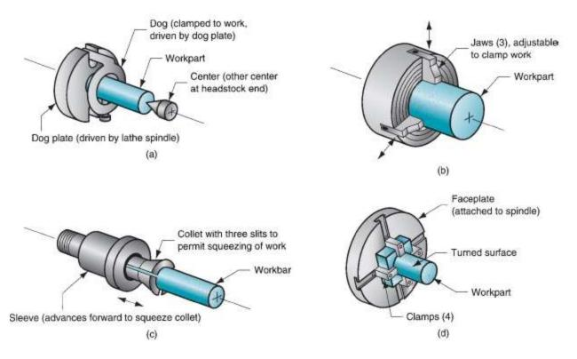
FIGURE 9.8 Four workholding methods used in lathes: (a) mounting the work between centers using a dog, (b) three-jaw chuck, (c) collet, and (d) faceplate for non-cylindrical workparts.
