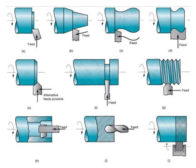
FIGURE 9.6 Machining operations other than turning that are performed on a lathe: (a) facing, (b) taper turning, (c) contour turning, (d) form turning, (e) chamfering, (f) cutoff, (g) threading, (h) boring, (i) drilling, and (j) knurling.
