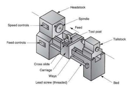
FIGURE 9.7 Diagram of an engine lathe, indicating its principal components.
