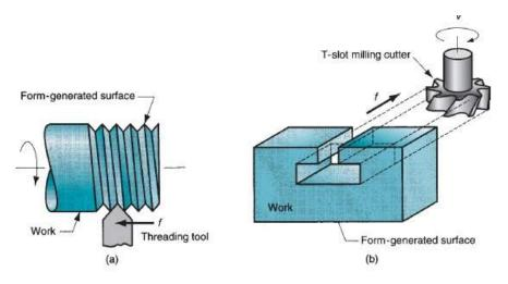
FIGURE 9.4 Combination of forming and generating to create shape: (a) thread cutting on a lathe, and (b) slot milling.
