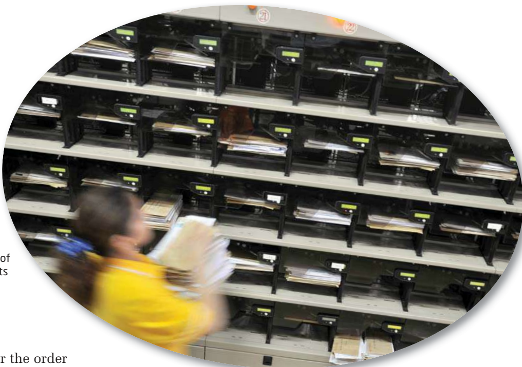
Sorting by hand mail that has been rejected by the machine sort due to unrecognizable hand-written or missing postal codes
