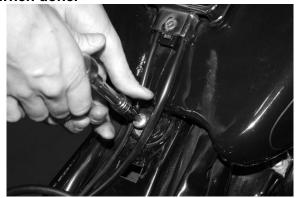
Remove rear tank bolt
