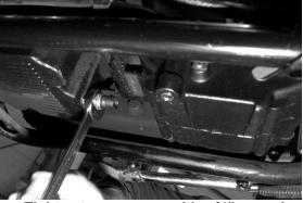
Tighten temp sensor with a 3/4" wrench
