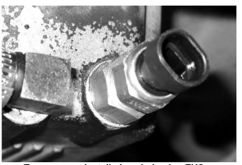
Temp sensor installed as drain plug EVO
