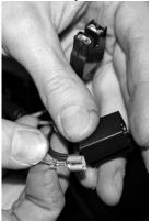
Remove the pin from the connector
