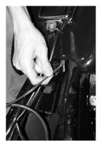
Route wires under tank Pull the temp sensor wires through the fairing
