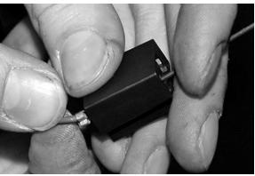
Using a small allen/pick release the locking tab
