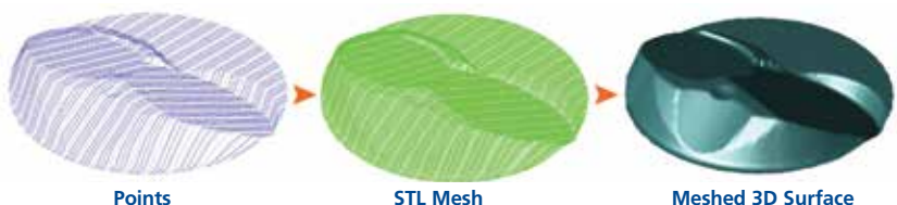
Piston Head – Reverse Engineered
