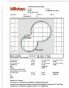
The contour compared to the nominal "AS IS." The areas shown in red fail to meet the profile requirement.
