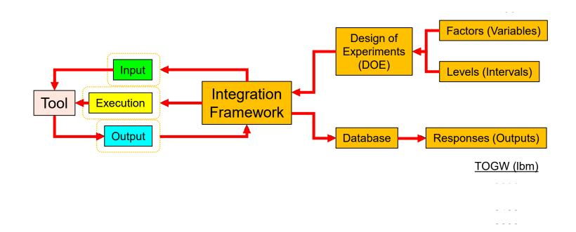
Once the design process is automated, this enables Design Space Exploration with a variety of Design of Experiments (DOE) techniques
