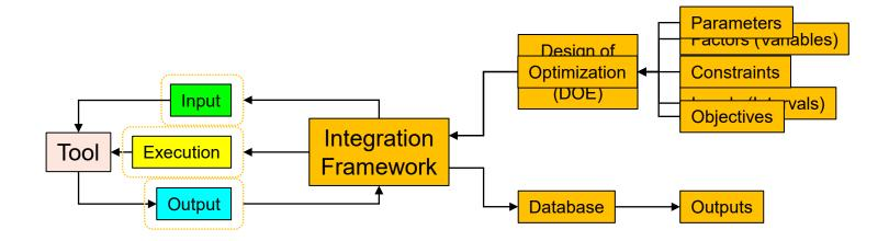
Once the design space has been explored, a variety of Optimization techniques may be applied to find local/global maximums and minimums of some specified objective function, subject to given constraints, in the design space
