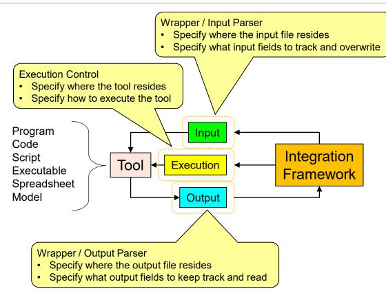
Once integrated, the tool is considered "wrapped" and can be executed automatically by the Integration Framework
