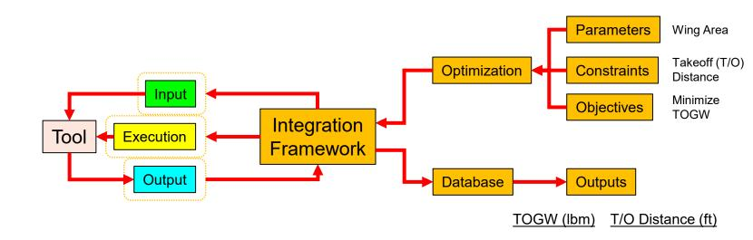
Once the design space has been explored, a variety of Optimization techniques may be applied to find local/global maximums and minimums of some specified objective function, subject to given constraints, in the design space
