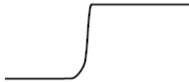
Signal with a short ground lead
