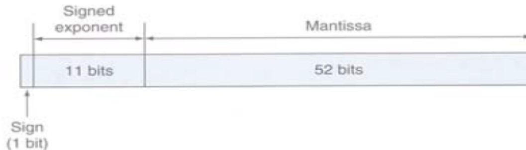
Figure: The manner in which a floating point number is stored in IEEE double precision format
