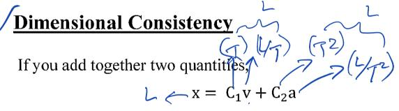
these quantities need to have the same dimensions (units); e.g., if x, v and a have units of (L), (L/T) and (L/T<sup>2</sup>), then  $C_1$  and  $C_2$  must have units of (T) and T<sup>2</sup> to maintain dimensional consistency.
