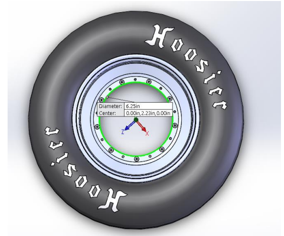
Figure 52: Maximum Diameter of Caliper Assembly as Determined by 10" FSAE Tire
