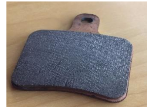
Figure 57: Sintered metal pad that was donated by Hayes performance systems
