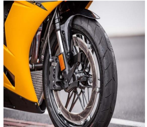
Figure 55: EBR 1190 front caliper features an inverted geometry similar to what Wisconsin Racing is attempting
