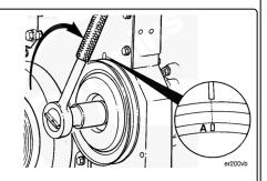
When the "A" mark is aligned with the pointer, the intake and exhaust valves for cylinder Number 1 **must** be closed. If these conditions are **not** correct, cylinder number 6 injector and
