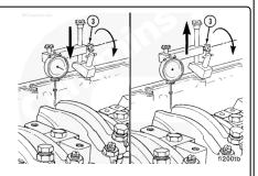
Actuate the injector plunger three or four times to remove the fuel from the injector assembly. Allow the lever to return slowly to prevent damage to the dial indicator.
