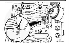
Apply a non-chlorinated carburetor cleaner (Pyroil®, or equivalent). Use a narrow bore orifice or extension tube of 2 mm [0.079 in] maximum outside diameter (O.D.), into the injector weep hole.
