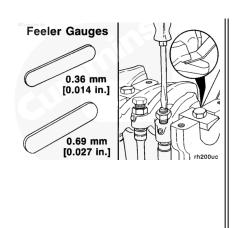
Insert the feeler gauge between the top of the crosshead and the rocker lever pad.
