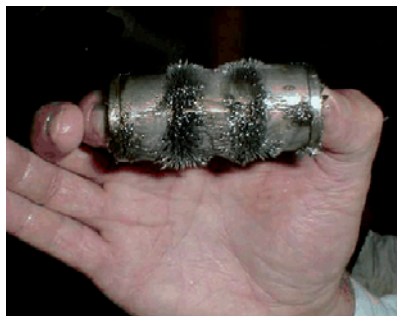
Fig. 1: Magnets can be used to detect contamination of oil through metal particles.
